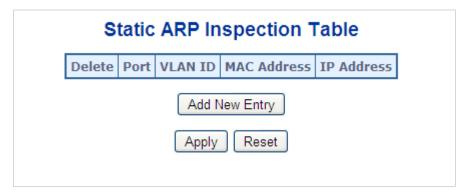
Figure 4-5-10-2: Static ARP Inspection Table Screen Page Screenshot
