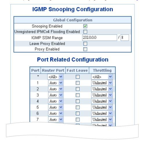
Figure 4-3-5-7: IGMP Snooping Configuration Page Screenshot
