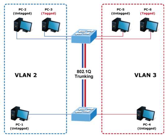
Figure 4-3-3-11: VLAN Trunking Diagram
