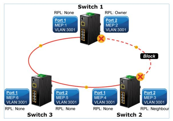
Figure 4-7-6: Ring Example Diagram
