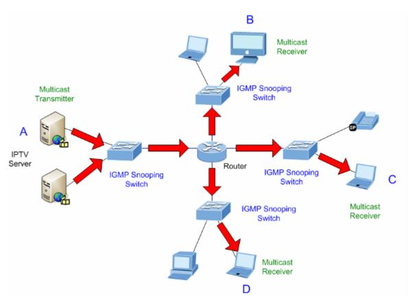
Figure 4-3-5-3: IGMP Snooping Multicast Stream Control
