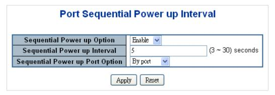
Figure 4-6-6-1: PoE Port Sequential Power Up Interval Configuration Screenshot
