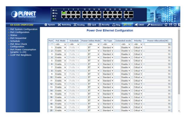
Figure 4-6-1 Power over Ethernet Web Screen
