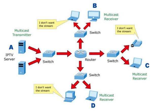
Figure 4-3-5-2: Multicast Flooding
