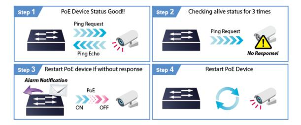
This page provides you with how to configure PD Alive Check. The screen in Figure 4-6-7 appears.
