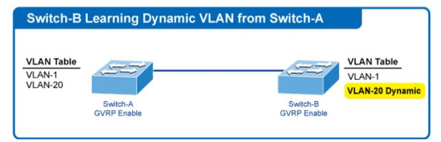
VLANs are **dynamically** configured based on **join messages** issued by host devices and propagated throughout the network.
