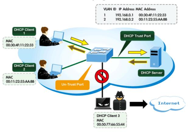
Configure DHCP Snooping on this page. The DHCP Snooping Configuration screen in Figure 4-5-6 appears.
