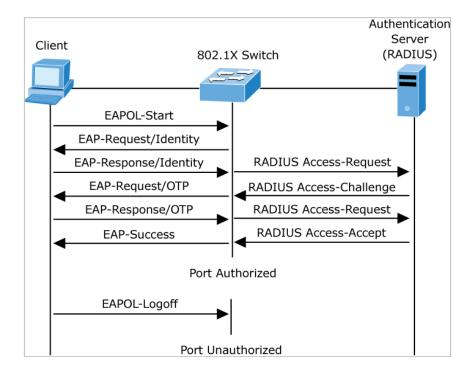
Figure 4-5-2: EAP Message Exchange
