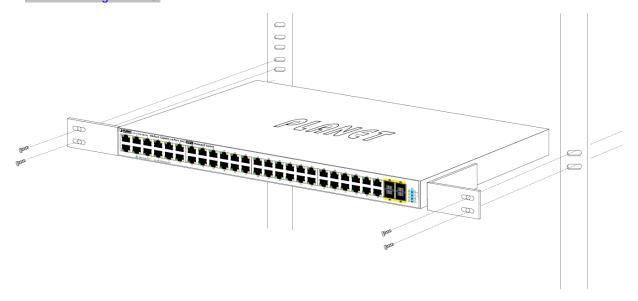
Figure 2-2-3: Mounting Managed Switch in a Rack
