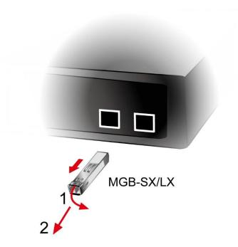
Figure 2-2-5: How to Pull Out the SFP/SFP+ Transceiver
