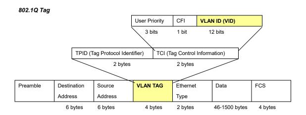
The Ether Type and VLAN ID are inserted after the MAC source address, but before the original Ether Type/Length or Logical Link Control. Because the packet is now a bit longer than it was originally, the Cyclic Redundancy Check (CRC) must be recalculated.
