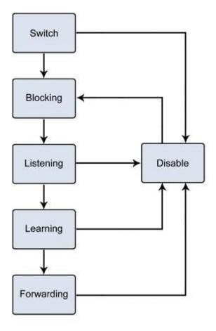
Figure 4-3-4-1: STP Port State Transitions
