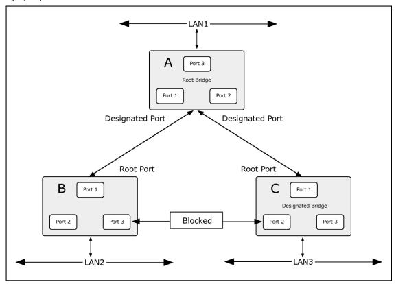
Figure 4-3-4-3: After Applying the STA Rules
