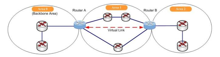
Following is OSPF virtual link configuration table. The virtual link is established between 2 ABRs to overcome that all the areas have to be connected directly to the backbone area. The screen in Figure 4-10-5-8 appears.
