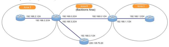
Following is OSPF area configuration table. It is used to specify the OSPF enabled interface(s). When OSPF is enabled on the specific interface(s), the router can provide the network information to the other OSPF routers via those interfaces. The screen in Figure 4-10-5-2 appears.
