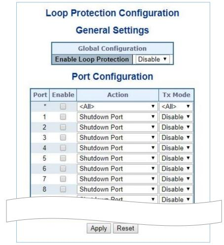
Figure 4-3-10-1: Loop Protection Configuration Page Screenshot
