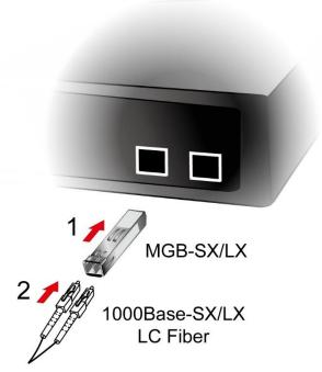
Figure 2-2-4: Plug-in the SFP/SFP+ Transceiver
