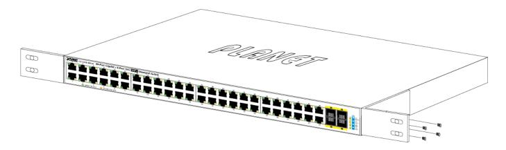
Figure 2-2-2: Attach Brackets to the Managed Switch.
