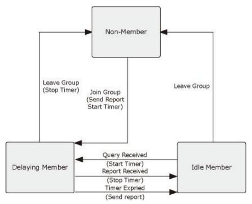
Figure 4-3-5-4: IGMP State Transitions
