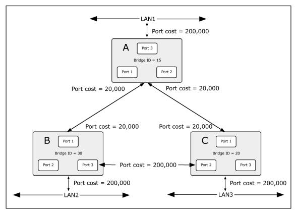
Figure 4-3-4-2: Before Applying the STA Rules
